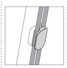
A cord management system allows different power and data cords to easily be secured on each leg.
