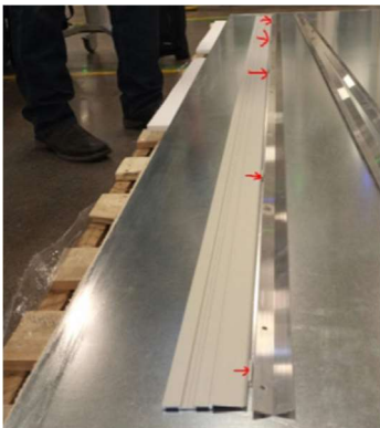
Figure 4: The new hanger bar will sit flush against the spacers installed.
