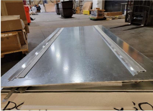
Figure 3: Back of whiteboard is to be cleaned with alcohol wipes where new hanger bar will be mounted.
