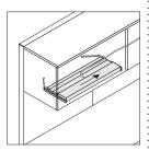
**Shelf light** can be mounted anywhere from side to side beneath over-head storage bin or shelf. The cord length is the only limitation.
