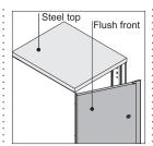
Steel top is standard on lockers with steel door fronts. Optional laminate or veneer tops are available on all lockers. All proud door fronts overlap the steel top.
