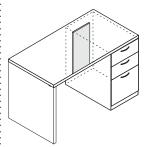
1. Single pedestal desks less than 48"W require a counterweight. Single pedestal desks with 30"D pedestals require a counterweight.
