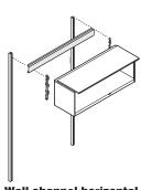
Wall channel horizontal brace is required with wall channels to support bins that are wider than 48".
