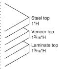
Laminate and wood veneer tops with squareedge profiles are available in place of standard 1"H steel tops. Laminate and wood veneer tops are 3/16" taller than steel tops and will add that dimension to the overall height of the lateral file.
