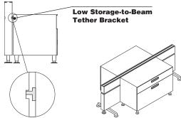
3. Counterweights are not required for 1.5-High lateral file or low storage tethered to a c:scape beam when the storage is the same size and mirrored back-to-back on both sides of the beam.
