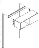
Wall channel horizontal brace is required with wall channels to support bins that are wider than 48". Page 64
