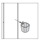
Peg is available as an option when markerboard finish is selected on back panels. Peg is installed at 36" above finished floor and 31/2" inboard from outside face of cladding.
