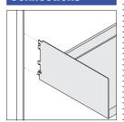
Steel support hooks on end supports insert into the slotted channel of a panel or wall channel and lock into place with a safety catch.
