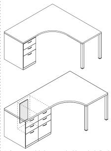
5. A counterweight is not required for a single fixed pedestal attached to desks made with corner, extended corner, or 120° corner worksurfaces. Any additional pedestals within the application require counterweights.
