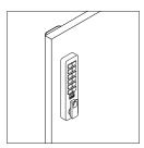
Electronic locks are Digilock Versa keypad locks and are powered by two lithium 2450 batteries. Tip: When electronic lock option is selected, the pull option cannot be selected. Electronic locks replace the pulls on doors.
