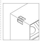
**Soft-touch integral handle on mobile unit** allows for easy movement from one location to another.
