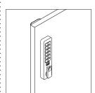
Locks come set to shared use mode. The user locks with a 4-7 digit code and unlocks with the same code. Once unlocked, the lock is reset for another user.
