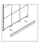
**Plinth covers** span multiple lockers and have a horizontal grain direction.
