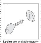
or field-installed. Factoryinstalled locks are standard and available keyed random only. Optional field-installed locks are available with consecutive, specific, and random keying options. Master-keyed locks are also available. Field-installed lock cylinders must be specified separately.
