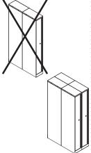
Lockers can be ganged in back-to-back applications only if there are a minimum of four lockers-two side-toside and two back-to-back.
