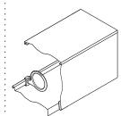
**Back of storage bin** is open to allow panel surface to show. Metal backstop prevents contents of bin from damaging panel surface.
