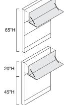
Overhead storage shelves install at 65"H only. They cannot install on a 10"H stacker or any base frame lower than 65"H Tip: A special half-height shelf is available, contact Systems Specials Group for an engineering quote.
