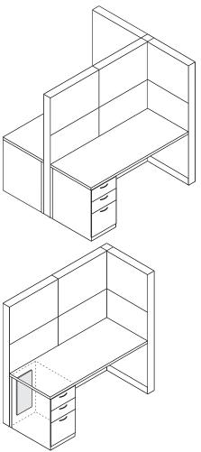
Counterweights are not required for fixed pedestals installed below a worksurface attached in a panel spine application. Single workstation applications **require** a counterweight in each pedestal.
