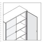
Frosted glass hinged doors are available as an option on all bookcases. Glass doors do not lock. Pulls on glass doors are available in four finishes. Doors ship separately from the bookcase and are field-installed.
