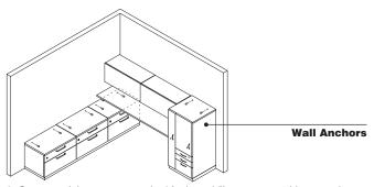
2. Counterweights are not required for lateral files, towers, cabinets, and bookcases anchored to the wall.
