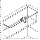
**Dividers** are available as an option for use on bins. Dividers ship in a package of four.
