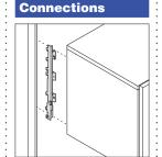
Steel support hooks on end supports insert into the slotted channel of a panel or wall channel and lock into place with a safety catch.
