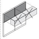
**Two bins** cannot be hung side by side if one or both bins are in front of a slatwall skin.
