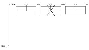
For Bottomline lights, starter light is required with daisy chain lights to bring power to the first light in the
