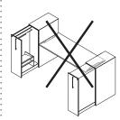
Worksurface support bracket can be used to support one side of a worksurface only.
