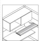
**Shelf lights** are available for use beneath bins. Lights recess into the bottom of the overhead storage unit.
