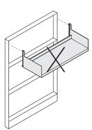
**Overhead storage** components cannot be attached to Montage frames with glass tiles.
