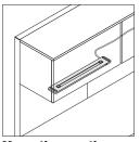
**Magnetic mounting** allows shelf light to be installed without tools under most metal overhead storage bins and shelves. This mounting allows the light to be mounted to most competitive steel bins and shelves.
