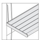
**Gap at back of slim shelf** allows routing of shelf light cord.
