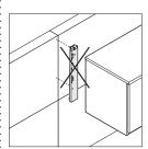
Horizontal off-module brackets cannot span a vertical or joint where two frames come together on enhanced off-module Montage panels. Shift the bin to avoid the joint.
