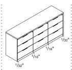
1/16" is added for space between each unit plus an additional 1/32" on each end. Example: Three 30"W units would have 903/16" interior width.
