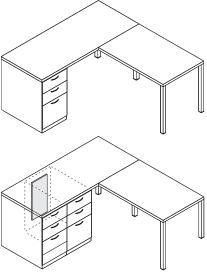
4. A counterweight is not required for a single fixed pedestal attached to a desk attached to another worksurface in an L-configuration. Any additional pedestals within the application require counterweights.
