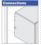
Steel support hooks on end supports insert into the slotted channel of a panel or wall channel and lock into place with a safety catch.
