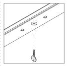
Lock in bin is concealed from view beneath the shelf. Locks are available factory or field-installed. Factory-installed locks are standard and available keyed random only. Optional field-installed locks are available with consecutive, specific, and random keying options. Master-keyed locks are also available. Field-installed lock cylinders must be specified separately.
