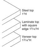
Steel, laminate, and wood veneer tops are available in place of standard 1/8"H steel tops. 1"H steel tops, 13/16"H laminate with square edge profile, and 13/16"H wood veneer with square edge profile.
