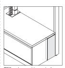
**Filler** is used in end-of-run applications where end of storage unit will be visible.
