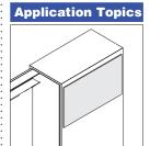
Magnetic boards, available as an option, are fabric-wrapped steel providing a place for visual display. The size of the magnetic board is determined by high-density case height and depth. Magnetic boards are field installed. Tip: Magnetic board is not
