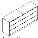
Sectioned tops are optional based on the width of the top. One- to four- sections are allowed between specific ranges that can be realized through SmartTools.
