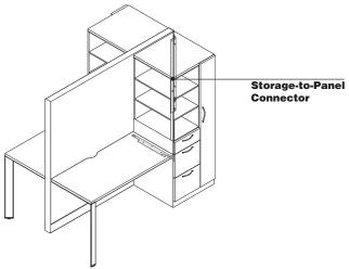
4. Counterweights are not required for towers used with a storage-to-panel connector to support the panel run, if the application is mirrored back-to-back (a two-pack minimum) and the panel is equal to or greater than 5'.
