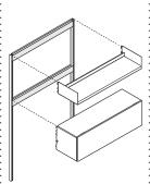
**Wall channel horizontal** brace is required for EACH storage bin or shelf that is wider than 48". The brace should be placed at the position along the vertical wall channel where the top of the bin or shelf will be placed.
