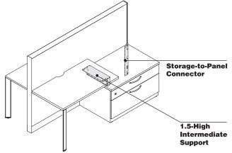
3. Counterweights are not required for One-High, 1.5-High, and Two Drawer lateral files and cabinets used with a storage-to-panel bracket to support the panel run if the application is mirrored back-to-back (a two-pack minimum) and the panel run is equal to or greater than 6'.
