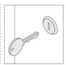
Locks are available factory or field-installed. Factory-installed locks are standard and available keyed random only. Door and drawers are keyed alike. Optional field-installed locks are available with consecutive, specific, and random keying options. Master-keyed locks are also available. Field-installed lock cylinders must be specified separately.
