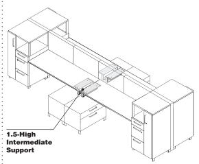
2. Counterweights are not required for One-High and 1.5-High lateral files and cabinets used with an intermediate support, when the application is mirrored back-to-back (a two-pack minimum).
