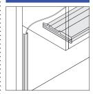
Wire manager is available for use between the bottom of a shelf or overhead storage bin and a worksurface. Wire manager can be cut in the field to suit specific application.
