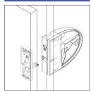
Lock mechanism is attached to inside of the locker opening and a flexible bolt is attached to the door. Bolt is secured in the mechanism when lock is in use.
