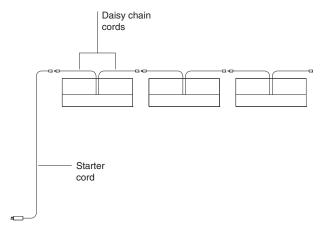
Power will not be interrupted in a chain even if one of the shelf lights is turned off or its lamp has burned out. That's because the path of power through the chain doesn't pass through the lamps or switches.
