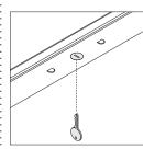
Lock in bin is concealed from view beneath the shelf. Locks are available factory or field-installed. Factory installed locks are standard and available keyed random only. Two-door units are keyed alike. Optional field installed locks are available with consecutive, specific, and random keying options. Master-keyed locks are also available. Field-installed lock cylinders must be specified separately.
