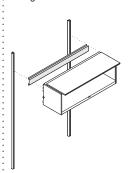
Wall channel horizontal brace is required with wall channels to support shelves and bins that are wider than 48".
