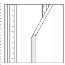
**Flush-front pull** is full height and integral with the door. Pull is available on steel doors only.
