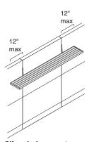
Slim shelves can be mounted off-module. No more than 12" overhang on either side of panel is recommended. Brackets attach on vertical seams of panel, while the shelf adjusts off-module on the brackets.
