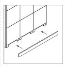
**Plinth base** is required when specifying networked locks. Plinth cover, specified separately, conceals openings in plinth base providing a clean aesthetic.
