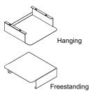
Personal shelf is specified in one of two ways. When specified as an option, the shelf is intended to install hanging from the top of the locker opening. When specified as freestanding, a separate style number is used
