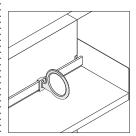
**Dividers** are available field installed for use on Universal shelves. Dividers ship in a package of four. Dividers cannot attach to Universal personal shelves.
