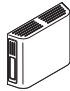
Enclosed CPU holder provides for an increased level of security for the CPU. Enclosed CPU holder is 4"D x 15 3/4"W x 12 1/8"H. Maximum recommended wattage of CPU is 396 watts.
