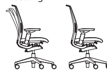
Mid-back stop recline setting Upright back stop setting
