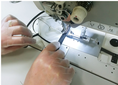
5C. Sew perimeter around entire circumference.
