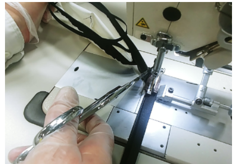
5C. Sew perimeter around entire circumference.
