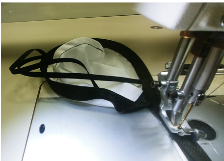
5D. Sew 1" extended strip off end (at startpoint) and trim.
