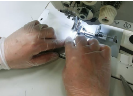
3B. Sew over existing seam as inside out, entire curved seam at 3/8" seam.
