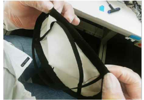
6B. Feed wire through tunnel until end is fully into tunnel – between top strap connection points.
