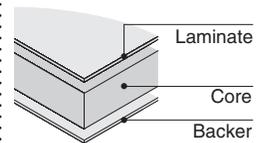
Solid core tops with 1/2" nominal edge thickness have a particle board core (45 lb cu ft density) with High-Pressure Laminate or wood veneer on the top and a backer applied to the opposite side for a balanced construction. High-Pressure Laminate, wood veneer, and backer are bonded to the core with a PVA adhesive.
