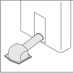
Floor monument kit should be specified when above-the-floor monument is used or when a flush floor monument is not positioned under a base. Above-the-floor monuments may not fit inside a base. Oval conduit is 4 1/5" x 2"H. The floor monument is 6 1/5"L x 7 1/2"W x 3 3/8"H.
