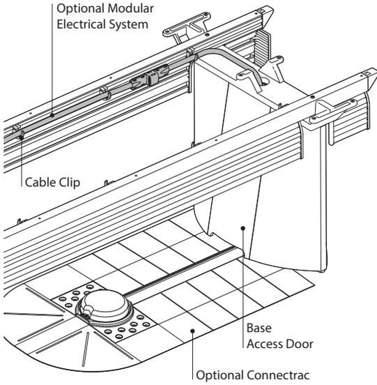
If **optional modular electrical system** is specified, bring wiring up through base from floor monument or base access door into Tech Corridor. A hardwire infeed is used for the modular electrical systems. For single TAP styles, the modular infeed is not needed. Specify the hardwired tray option. Connect electrical cables and secure with cable clips. Run data wires along opposite beam and secure with cable clips as required.
