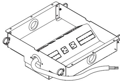
**Hardwired tray** will have a 6' conduit and a three-wire hardwire connection.
