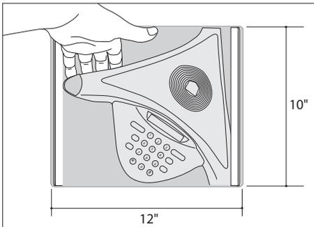
**Table top opening for storage tray** is 12" x 10", trimmed with a flat solid wood profile. Two doors conceal access to a black powder coated steel tray that can house equipment, such as most common speaker phones. The inside dimensions for the storage tray are 15<sup>7</sup>/<sub>8</sub>" x 13<sup>3</sup>/<sub>4</sub>" x 2<sup>13</sup>/<sub>16</sub>".
