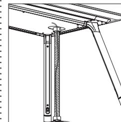
**Cutouts in the bottom tray** provide an alternate way to route cords and cables to and from tables using a cable manager. Cutouts are located on end and center locations and measure: 24"D tables, 2 1/2" x 4 23/32"; 30"D and 36"D tables, 3 1/2" x 5 1/8".
