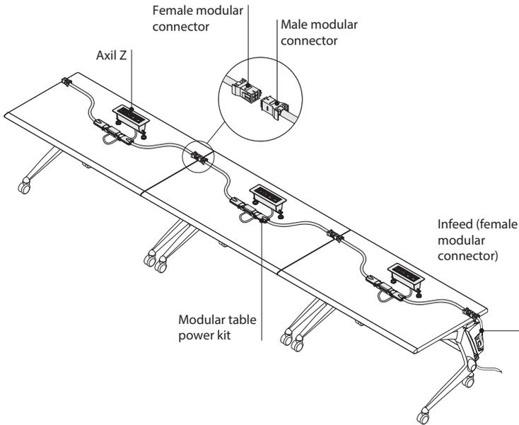
The duplex receptacle(s) in the table power kit and every two simplex receptacles from the desktop module count against the 13 duplex receptacles allowed for each circuit. The above example has a total of nine duplex receptacles being utilized.
