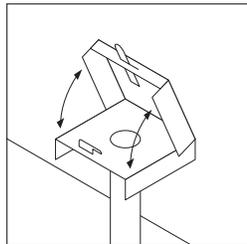
**Flip-top mechanism** is available on pedestal base tables 36"D or less. The flip-top mechanism allows tops to tilt for more compact storage of tables that are not in use. Safety latch secures the top in flat position and must be released to flip top up.
