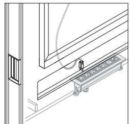
The monitor for the mobile mediaboard display will be routed to plug into the power module in the well. The remaining simplex outlets are used to power up to four mobile devices, including laptops and iPads.
