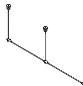
**When two power module units are specified**, they are connected by a corded system and have a single infeed with a 15-amp plug. After exiting the leg, there is at least 60" of cord length available to connect to power source.
