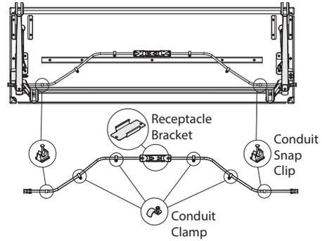
1. Identify the conduit path along the center channel. Utilize predrilled holes in the surface for all components. *Note: Conduit on 24"W Tables will "jump" the center spine (as shown). Conduit on 30"W tables will be located to the rear of the center spine.*
