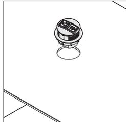
Round power module is only available on round and square tables and is centered. The 3" module is available in silver, milk, black, and graphite finishes. It comes with a 8'L power cord with 15-amp plug. Plug includes a built-in circuit breaker measuring 2¼"D x 1½"W x 1½"H. Round power module is available with two simplex receptacles or one simple/2 USB charging ports. USB receptacles conveniently charge a range of electric devices. Some devices may not be compatible.
