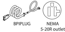
**Single circuit plug**, 20-amp, base power-in, 3+0 wiring schematic is available on tables with one, two, three, or four utility bays. This offers the quickest, easiest installation of tables. An electrician must provide a NEMA 5-20R outlet for each row within 18" of the infeed location. The single circuit plug is U.L. recognized.
