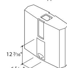
**Veneer base** is hardwood veneer on MDF. Wood veneer surfaces are available in all Coalesse standard species and finishes. The removable access door, 6 5/16"W x 12 7/16"H, is secured with a reclosable fastener. Veneer bases are available in two sizes, 24"W and 30"W. Bases have glides adjustable up to 1/2" (providing a total floor clearance of 3/4").
