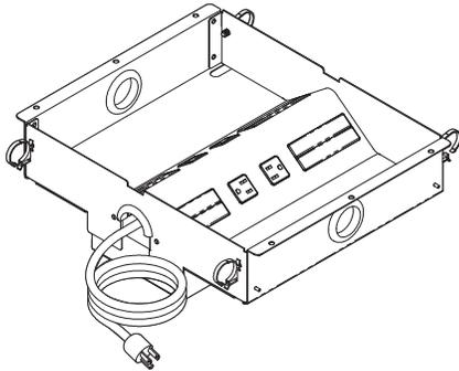
**Cord and plug tray** will have a 10' cord and 15-amp plug. Each TAP tray must be plugged into a floor outlet. This TAP tray cannot be daisy-chained.
