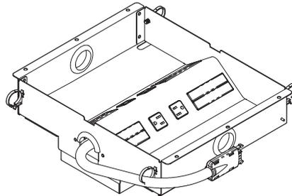
**Modular tray** will have a modular harness that "daisy-chains" from one TAP to the next. A two-circuit, four-wire hardwire base power infeed is included.
