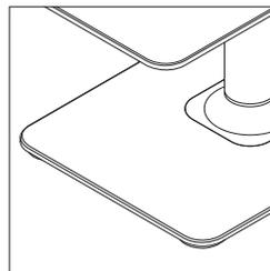
**Non-adjustable 3" diameter plastic glides** are standard on all tables. Glides are ⅜" thick for the 36"D x 72"W table; ½" thick for all other work and occasional tables; and ¼" thick for the personal table. For all work and occasional tables the glide height is needed to route cords.
