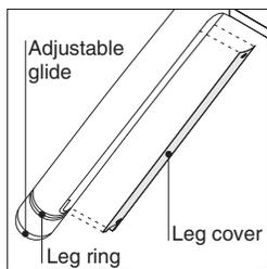
**Removable cover on metal leg** allows easy access and installation of technology cords.
