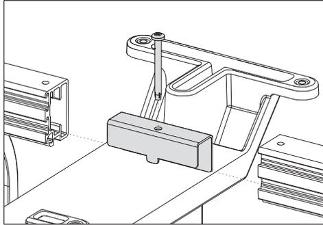
**Align black rail clamps** with predrilled holes in center base bracket casting. Position each clamp with the tab pointing downward, and the short side of the clamp facing inward.
