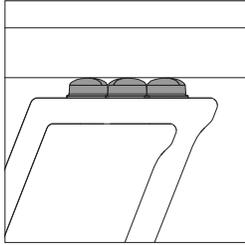
**Glass tops** rest directly on rubber bumpers attached to the base and are available in two tinted, acid-etched finishes. The glass is 1/2" thick.
