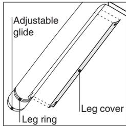
Removable cover on metal legs allows easy access and installation of technology cords.
