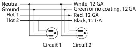
The modular table power kit is a 20-amp, 4-wire, 2-circuit system. Each circuit allows up to 13 duplex receptacles. The 20-amp plug infeed only allows up to 13 Circuit-1 duplex receptacles, and the hardwire infeed allows up to 26 Circuit-1 and -2 duplex receptacles, no more than 13 per circuit.
