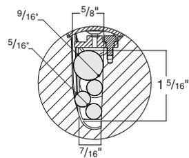
**Cross-section view** showing conduit and cable routing capacity through the leg. Every metal leg has cable routing capability.
