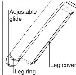
**Cable routing** is accommodated through the metal legs and can be accessed through the removable cover.
