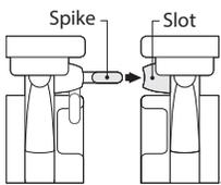
A coupling device is built into every Train Table to enable tables to gang together end-to-end without tools or separate parts. All Train tables that have modular table power specified, requires the tables to be connected with the coupling device provided.
