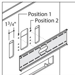
In order to install the monitor mount bracket, the back panel must be removed. Use the provided bolts and install to the desired mounting hole position on any mobile mediaboard unit. The front panel also has cutouts to route the wires from the monitor for a clean aesthetic. Top hole for position 1 is 1 3/4" from top. Position 2 is 1 3/4" lower.
