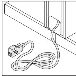
The corded plug on the power and display module is a 15-amp plug with a circuit breaker on the end. The cord has approximately nine feet of extension from the grommet exit point.
