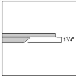
**Solid surface and glass tops** are built with a substructure (bottom) and top construction. The substructure is 1 1/4" in thickness and is available in black or white. The glass or solid surface top is 1/2" thick. *Tip: Glass tops are not secured to the substructure. Glass tops are placed on rubber pads that are adhered to the substructure. If the glass tables need to be moved, remove the glass top prior to moving the table.*
