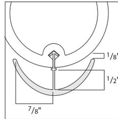
The vertical wire manager is divided into two sections for cord and cable management. Three cords/cables can be routed per section.
