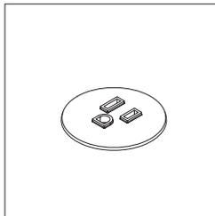
**Single power or USB module** are available and can be specified in end or center locations. It comes with a 120°L power cord with 15-amp plug. The USB module has one USB A and one USB C 5V charging port. After exiting the leg, there is at least 30" of cord length available to connect to power source. If a single USB module is specified, the 15-amp plug includes a built-in transformer measuring 2 1/8"D x 1 1/4"W x 3 1/2"H. The power modules are available in milk, black, or graphite.
