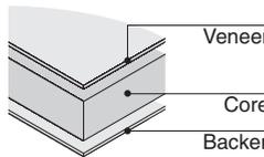
**Wood veneer table tops** are fabricated with Architectural Grade AA hand-selected hardwood veneer, plain sliced, book matched, and bonded to the core with a backing sheet for balance. Coalesse's primary wood finish, Clarity, is a waterborne UV topcoat, which protects the environment while providing exceptional durability and resistance to water and chemical stains. Due to natural variations in wood, finished products may vary from samples in color, texture, and grain.
