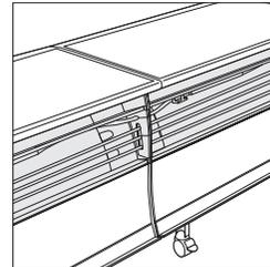
Raceway includes a 3" x 6" interior cavity that can accommodate approximately 40 four-pair UTP cables. Wire guide in this space is a steel bracket with numerous holes suitable for wire ties or clips to support tidy wire management. Raceway end caps have flexible vinyl openings to allow lay-in cable routing. Cables can enter or leave the raceway through openings in the valance panel.
