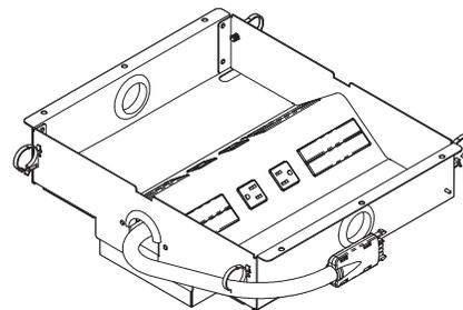
**Field-wired tray** will have two single-gang faceplate openings for customer's own power outlets and wiring.
