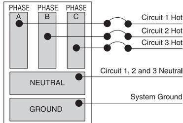
On a single 3-phase circuit panel, all three circuits are distributed as shown.
