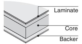
Solid core tops with 1" nominal edge thickness have a particle board core (45 lb cu ft density) with High-Pressure Laminate and a backer applied to the opposite side for a balanced construction. High-Pressure Laminate and backer are bonded to the core with a PVA adhesive.
