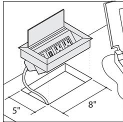
Ellora is an 8 1/4" x 5 1/4" desktop module that mounts at the top surface of the table and can be configured in several choices of power/data/USB:
