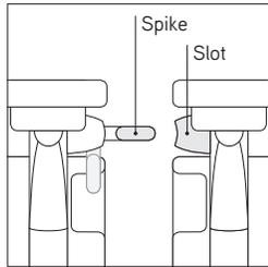
**Coupling device** is built into every Train table to enable tables to gang together end-to-end without tools or separate parts.
