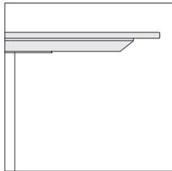
The table top is built into two sections, the substructure (bottom) and the table top. The substructure is a solid core of 45 lb median-density particle board, 1 1/4" thick, available in black or milk. The 1/2" thick top is available in the following:
