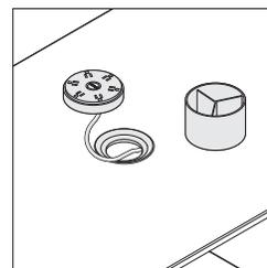
**The contour of the PowerPod bottom cradle** is designed to work in conjunction with the grommet for a snug fit.
