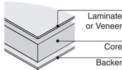
**Solid core tops with 1<sup>1</sup>/<sub>4</sub>" nominal edge thickness** have a particle board core (45 lb cu ft density) with High-Pressure Laminate or wood veneer on the top and a backer applied to the opposite side for a balanced construction. High-Pressure Laminate, wood veneer, and backer are bonded to the core with a PVA adhesive.
