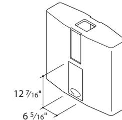
**Laminate base** has a laminate surface on molded fiberboard. The removable access door, 6 5/16"W x 12 7/16"H, is secured with a reclosable fastener. Laminate bases are available in two sizes, 24"W and 30"W. Bases have glides adjustable up to 1/2" (providing a total floor clearance of 3/4").
