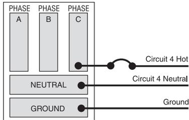
In the four-circuit, 3+1 schematic, circuits 1, 2, and 3 are distributed from the first circuit panel and are supported with one shared neutral and one shared ground. Circuit 4 is distributed from a second circuit panel and is supported with a separate neutral and ground.
