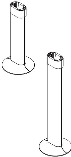
*Tip: This cable manager was designed to be used with the cut-outs in the bottom tray to manage cables from trough to floor.*
