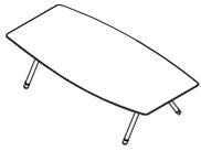
*Tip: Glass tops are not secured to the substructure. Glass tops are placed on rubber pads that are adhered to the substructure. If the glass tables need to be moved, remove the glass top prior to moving the table.*
