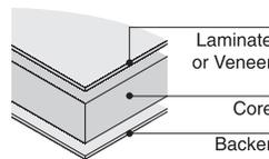
**Solid core tops with 1/4" nominal edge thickness** have a particle board core (45 lb cu ft density) with High-Pressure Laminate or wood veneer on the top and a backer applied to the opposite side for a balanced construction. High-Pressure Laminate, wood veneer, and backer are bonded to the core with a PVA adhesive.
