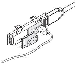
Duplex receptacles snap into power blocks on site. They are coded to indicate which circuit and type of ground they will engage. Tools are not required for installation. Tables that are 48" L can accommodate up to two receptacles. Tables that are 60" L or 72" L can accommodate up to four receptacles.
