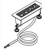
Axil Z hardware has six feet of flexible steel conduit for permanently hardwiring to the building power supply by a licensed electrician. This is to be used with tables with glides only, no casters. This version is best suited for municipalities where code requires hardwire connections for this type of desktop device or for installations where the furniture will not be reconfigured or moved.
