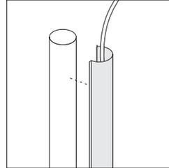
**Vertical wire manager** is available to clip on to Ballet table leg to conceal power cords and voice/data cables routed vertically from the floor to the worksurface. Vertical wire manager is black plastic. ▶ See page 45
