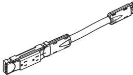
**Corridor power kit**, modular can be added only to modular trays. This kit adds two electrical outlets inside the tech corridor for plugging in speaker phones or other equipment that does not require frequent access.
