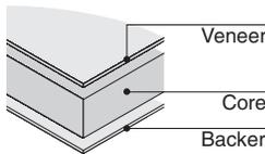
**Wood veneer table tops** are fabricated with Architectural Grade AA hand-selected hardwood veneer, plain sliced, book matched, and bonded to the core with a backing sheet for balance. Coalesse's primary wood finish, Clarity, is a water-borne UV topcoat, which protects the environment while providing exceptional durability and resistance to water and chemical stains. Due to natural variations in wood, finished products may vary from samples in color, texture, and grain.
