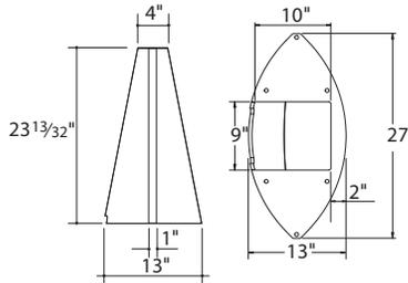
**Flared base** has a wood veneer surface on molded MDF with aluminum universal bracket. The removable access door, 9"W x 23 1/2"H, is secured with a ball catch fastener on each corner. Flared bases are available in one size, 13" x 27".
