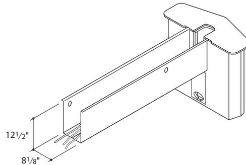
Beam assembly hangs from brackets attached to the bases and encloses all power and voice/data cables. Beam assembly consists of painted steel stretchers, side panels with a 1 1/2"-diameter access grommet on each panel, and a 4 1/2" wide raceway access door on the bottom of the raceway. Beams are 8 1/8"W x 12 1/2"H, with a capacity of 48 UTP cables.
