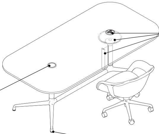
**Wire manager** comes standard with all power options and routes cords and cables from the cone to the floor. It is a separate piece that attaches to the column, available in black or milk. Additional wire manager options including cable tray are also available.
