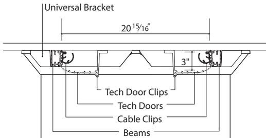
**Tech corridor** runs under the length of the table between the table top and the universal base brackets. Tech corridor creates a space approximately 20<sup>15/16</sup>" x 3" for cables, TAP tray(s), and optional equipment shelf(s).
