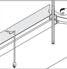
**Cable tray** can be attached to either side of central support beam on underside of surface.
