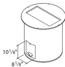
**Drum base** is molded MDF with either a laminate or a wood veneer surface. The removable access door, 8 1/8"W x 10 1/8"H, is secured with a reclosable fastener. The 24"-diameter drum base has a 12 1/2"-diameter opening in the bottom surrounded by a 60 lb weight for stability.
