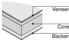
**Wood veneer table tops** are fabricated with Architectural Grade AA hand-selected hardwood veneer, plain sliced, book matched, and bonded to the core with a backing sheet for balance. Veneer tops and solid wood edge profiles are stained, and then finished with Coalesse's primary wood finish clarity, a water-borne UV topcoat, which protects the environment while providing exceptional durability and resistance to water and chemical stains.
