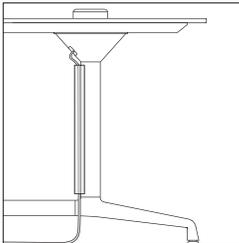
The SW\_1 vertical wire manager is supplied when a any non-hardwired power module is specified. It attaches to the groove in the base column to conceal and hold power cords and voice/data cables routed vertically from the floor to the worksurface. The wire manager is available in black or milk and automatically matches chosen subtop color. Note: For any occasional tables that can be specified with a PowerPod grommet or simple power unit, no vertical wire manager is supplied.
