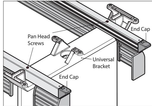
**Start the Pan Head screws** into each bracket casting. DO NOT tighten.
