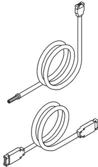
Power infeeds bring electrical power from the building to any table within a run of tables that are coupled together. Modular connections with the furniture is made at valance panel located at either end of the raceway on the knee-wall side, next to the table leg. Two alternative power infeeds can be used.
