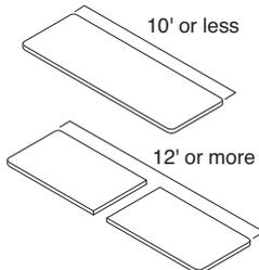
**Large tops** are shipped in sections with hardware for field assembly. Tops 12' and larger are shipped in two or more pieces.
