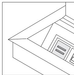
For Axil Z and Ellora, the USB for charging option is configured in the spot of one data port and is always configured on the end(s). It contains two USB ports for charging.
