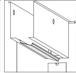
Wireway access door is placed in bottom of wireway. Flanges on top of door rest on side panel flanges.
