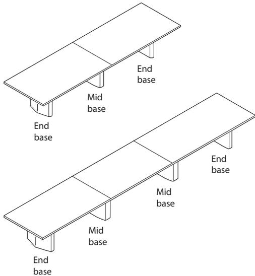
For tables 157"L and longer, you must specify the entry location for the base power of either "end base" or "mid base" entry location.
