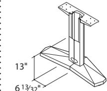
**Aluminum base** is cast and extruded aluminum, painted with Coalesse powder coat in any color. The black removable access door, 6 13/32"W x 13"H, is secured with screws. Aluminum bases are available in two sizes, 30"W and 36"W. Bases have glides adjustable up to 1/2" (providing a total floor clearance of 3/4").
