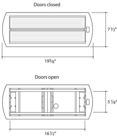
Utility bay is made of formed steel, painted gray, and houses power and data outlets. Overall, utility bay is 19 5/8"L x 7 1/2"W. Door opening is 16 1/2"L x 5 1/8"W.
