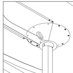
Cable tray is standard in platinum powder coat and attaches to the work surface between the legs, disguising the performance power module and ganged power system. The tray clearly routes wires and cables from the worksurface to the vertical wire manager or through the opening in the center of the tray, measuring 2" by 7/8" inches. The tray is available to specify on most rectangle and super-elliptical tables.
