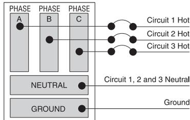
In the three-circuit, 3+0 schematic, circuits 1, 2, and 3 are distributed from the first circuit panel and are supported with one shared neutral and one shared ground.
