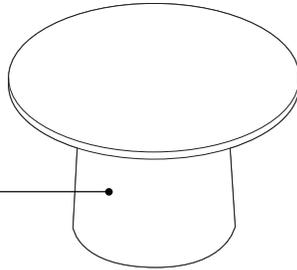
**Round base** is conical shaped plywood with wood veneer surface.
