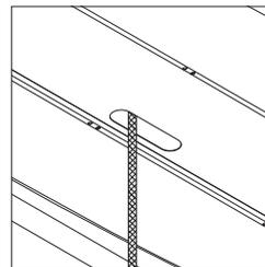
Mesh power cord cover is supplied when a power module is specified with hardwire infeed. The cover wraps around and conceals cords, allowing them to exit out of the center and down to the floor. The cover is black, measures 72" in length, and can accommodate up to 7/8" diameter of wiring. *Tip: Mesh power cord cover can be trimmed to the desired length.*
