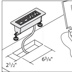
Axil Z is an 8" x 3" desktop module that mounts at the top surface of the table and can be configured in several choices of power/data/USB:
