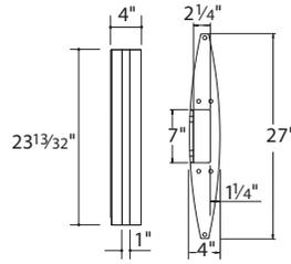
**Slim base** has a wood veneer surface on molded MDF with aluminum universal bracket. The removable access door, 7"W x 23 1/2"H, is secured with a ball catch fastener on each corner. Slim bases are available in one size, 4" x 27".
