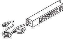
**Power strip** is available to provide additional power outlets beneath tables that must accommodate many technological components. Power strip includes six 15-amp outlets with surge protection, on-off switch, and 15' cord with three-prong plug. Power strip is black. UL and CSA listed and tested to UL standard 1449 at 400V.
