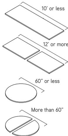
**Large tops** are shipped in sections with Tite-Joint fasteners for assembly on site. Table tops that are 12' and longer and table tops that are larger than 72" in diameter are always shipped in two pieces.
