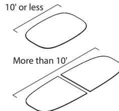
**Large tops** are shipped in sections. The 1/2" top and 1/4" bottom substructure are shipped separately and are assembled in the field. Tite-joint fasteners are used for the bottom substructure and other hardware is used to assembly the 1/2" top to the substructure. Tables that are 12' L and larger always ship in two or three pieces.
