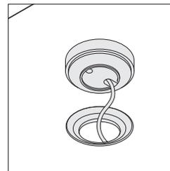
**PowerPod** is an option available on 30"D and 36"D tables. The grommet allows for pass through of cords and cables. The grommet is available in black or milk.
