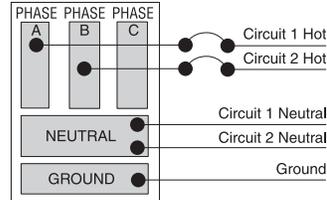
In the two-circuit, separate neutral schematic, circuits 1 and 2 are distributed from two different phases from the first circuit panel. Each circuit is supported with its own neutral and a common ground.
