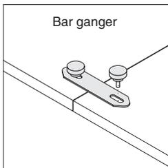
**Bar gangers** use steel bars to join adjacent tables. One end of the bar is captured by the host table and allows the bar to pivot beneath adjacent table where it is captured by a threaded post with knob. Factory-installed threaded insert in underside of table top accepts the threaded knob. No tools are required to link tables with bar gangers.
