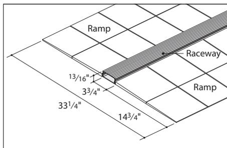
**Raceway interior**, 3<sup>1</sup>/<sub>8</sub>"W x 3<sup>1</sup>/<sub>4</sub>"H, provides ample room for wires and cable.
