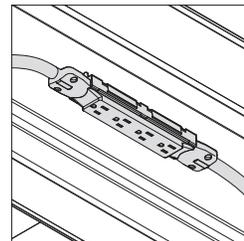
**A power harness** is concealed within the bottom tray and is specifically designed for each length of table. Drop in technology devices plug into the power harness.
