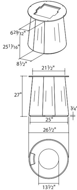
**Round base** is conical shaped plywood with a wood veneer surface, 26 1/2"-diameter bottom and 21 1/2"-diameter top. Underneath the round base is a 25"-diameter black painted wood inset, 3/4"H, with an opening. The 13 1/2"-diameter opening is surrounded by a 50 lb concrete weight for stability. The removable access door, 8 1/2"W at the bottom and 6.9"W at the top x 25 3/4"H, is secured with a ball catch fastener on each corner.
