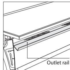
Outlet rail in the upper portion of the raceway has an opening to accommodate standard NEMA-style, single-gang, modular furniture voice/data faceplates.
