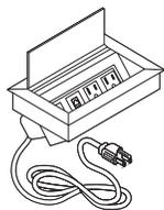
Ellora cord has a six-foot power cord and standard 15-amp plug for configurations with three or less simplex power outlets. The configuration of four simplex power outlets includes a non-standard 15-amp plug with a circuit breaker.
