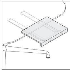
The tablets pull-out 10" from the worksurface and utilize two ball bearing slides.
