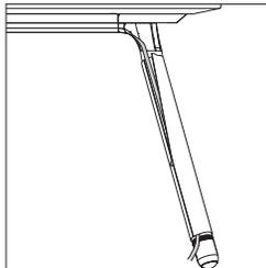
**Cables** can be managed down the wood legs with a cable management cover that zips around the leg. Cover is ordered separately and is available in a curated palette of Elmosoft leather colors for work and standing height tables.
