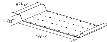
**Corridor shelf** is available to hold routers, hubs, line drivers, scalars and other technical equipment. Corridor shelf hangs between the beams and provides 1.5 rack units of space, 2<sup>3/4</sup>"H.
