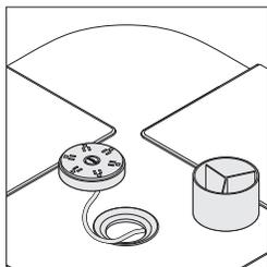
PowerPod grommet accommodates PowerPod or the pass through of cords and tables to the desktop. When specified, PowerPod grommets come with an inside barrier in the cone, and are available in milk and black finishes. PowerPod grommets can only be located above table legs (cone).
