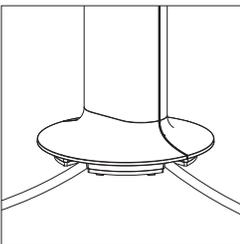
Cables can be concealed and run straight through the column to the floor, or out any side of the bottom, depending on location of building power supply.
