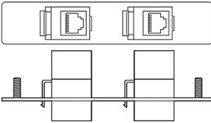
**Data Architectural Adapter Plate** has two CAT 5e RJ45 barrel (pass-through) outlets. It receives 2 plug-in at both ends of the barrel. Cat 5, 5e, and 6 will work with this coupler. The couplers must be 8-conductor type plug-ins on both ends.
