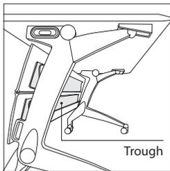
**Modesty panel** is available to enclose space beneath table and to provide two 2" x 3" wire management troughs. Panel is extruded aluminum with powder coat color to match the table legs. Trough is plastic extrusion. Modesty panel attaches to stretcher and swings open for access.
