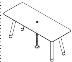
**The mesh cable manager** provides pass-through cable management and can be used with 30"D and 36"D Potrero415 light tables, with bottom tray specified. The mesh and steel components are black. The opening for cables measures 2" x 2 1/2".
