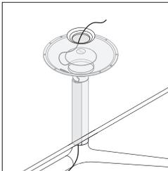
The cone at the top of the base attaches to the work-surface and accommodates the simple power module and PowerPod grommet. The cone allows cords and cables to be passed through and coiled for storage. If specified with PowerPod grommet, a barrier attaches to the inside of the column to help hold and conceal cords and cables. The barrier comes in black or milk to match the grommet.
