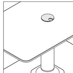
**A metal grommet** is an option on all work and occasional tables. The 3" grommet is flush-mounted and located in the center of the table top over the cone and column. The metal grommet is available in anodized silver only.
