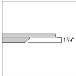
**Solid surface and glass tops** are built with a substructure (bottom) and top construction. The substructure is 1 1/4" in thickness and is available in black or white. The glass or solid surface top is 1/2" thick.
