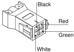
The modular connectors are color-coded for intuitive match-up when connecting the modular table power system. Match like colors only, i.e., green to green, red to red, black to black, and white to white.
