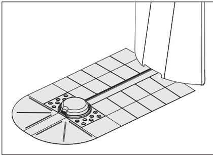
**Connectrac**, a floor monument kit, should be specified when a floor monument is not positioned under a base. Connectrac is a ADA compliant raceway that can be installed underneath carpet tiles or broadloom to conceal wires and cables running from a floor monument to the Host base.
