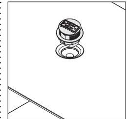
**Round power modules** are available on the focus nook, and all work and occasional tables. On the focus nook worksurface, the power module is specifiable on the back right or left side. On the tables, the power module is located in the center of the table top over the cone/column. The 3" power module features tamper resistant power simplexes, an 8'L power cord with 15-amp plug, and is available in four colors.
