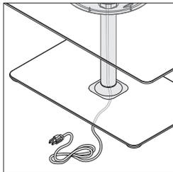
**Work and occasional tables** route cables and cords from the desktop through the column out through the base. Cords can be concealed in the cone.
