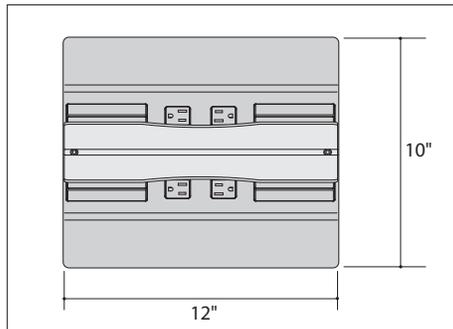
**Table top opening for TAP is 12" x 10"**, trimmed with a flat solid wood profile. Two doors conceal dual access to a black powder coated steel tray that houses power and data outlets.
