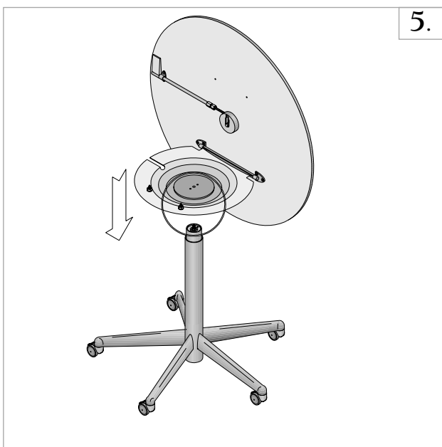
Position table top with understructure on the column.
