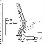
The core equalizer is powered by a torsional spring that adjusts with the angle of the seat and back to provide less lumbar support in a deep recline and more lumbar support in an upright posture.
