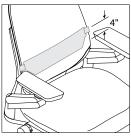
**Lumbar height** adjusts 4" (5<sup>1</sup>/4" to 9<sup>1</sup>/4") from seat by grabbing exposed tabs and sliding the lumbar support up or down. This feature is optional on work chairs and stools.
